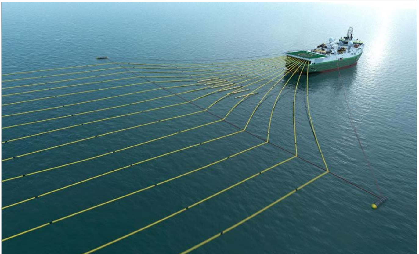
Figure 3. Example of a seismic array and marine seismic vessel for 3D or 4D surveys.
