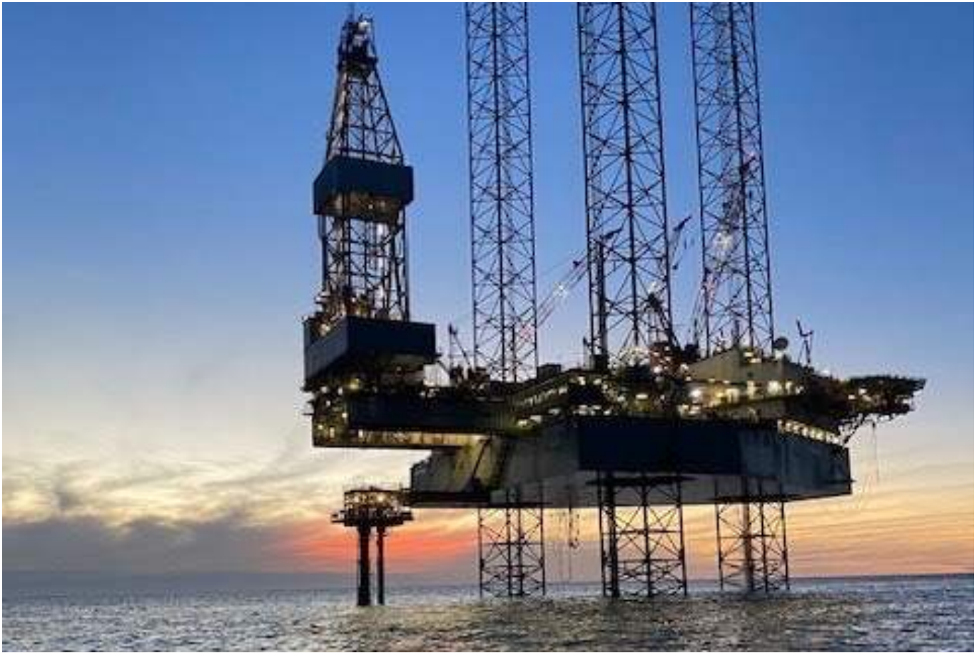
Figure 3. Example of jack-up MODU undertaking activities at a platform.
