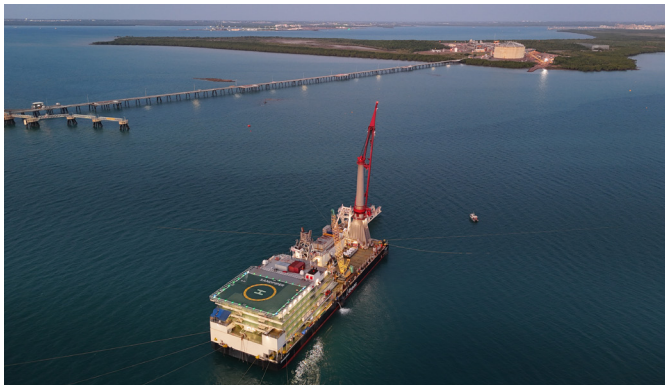
'Sandpiper' shallow water barge performing shorepull at DLNG
