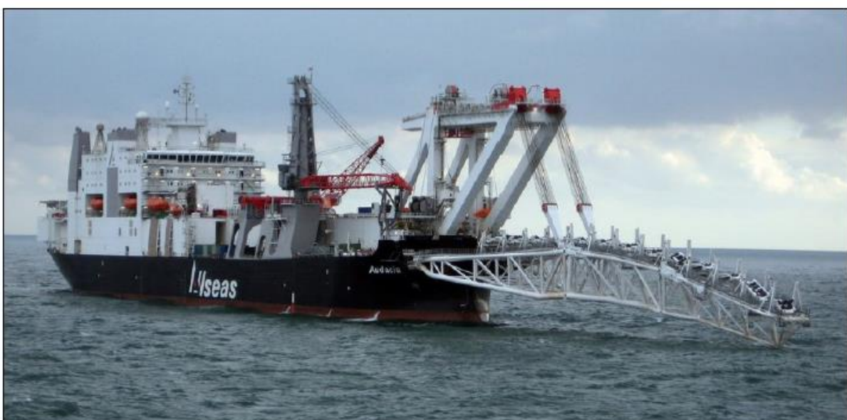
Figure 2-8 Example of pipelaying vessel (deep water vessel)
