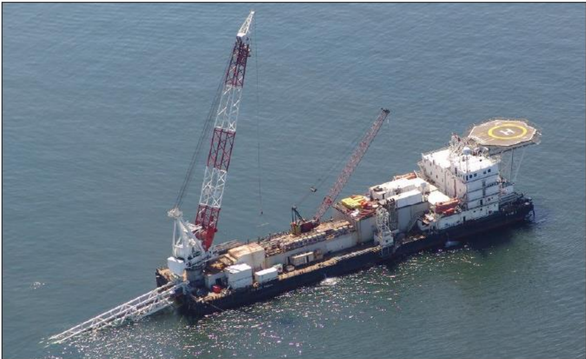
Figure 2-9 Example of pipelaying vessel (nearshore pipelay barge)
