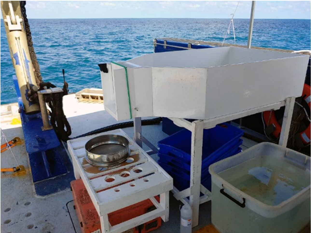
Plate 2-2: Infauna filtering table and puddling bin set up on the Lauri-J
