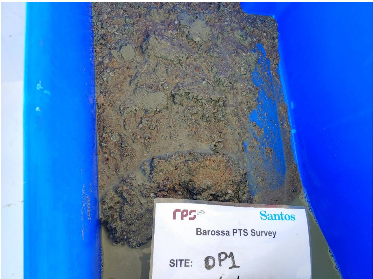
Plate 3-1: Grab sample from site OP1, showing silty shelly sand with clumps of clay
