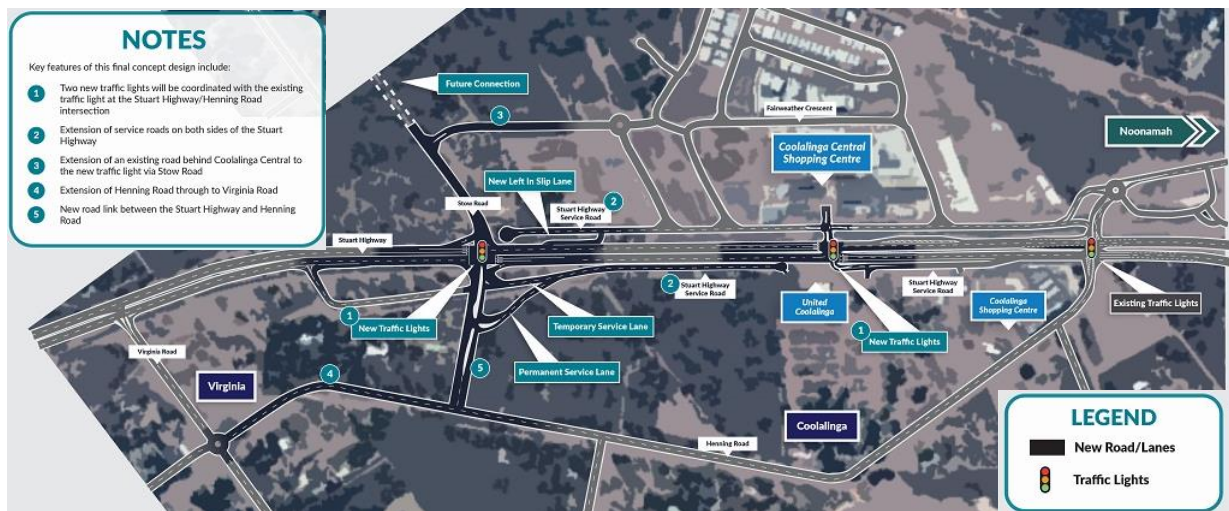
Figure 11-1: Coolalinga Road Safety Upgrades Plan
