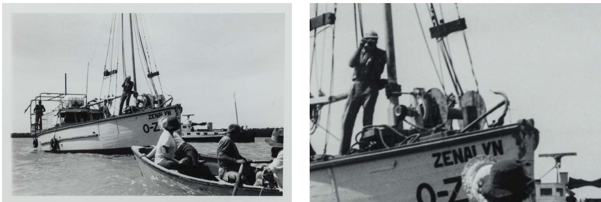
Figure 91: "Coastal trading vessel MV Zenalyn (ex-Catalina refuelling vessel) in Darwin Harbour." Note winch on foredeck (detail of winch on right). 115
