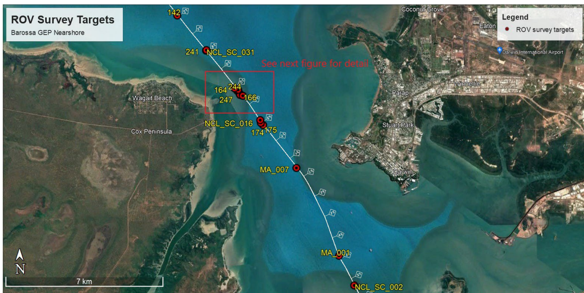
Figure 68: Location of ROV survey shortlisted targets. All targets located between KP 102 and KP 118.
