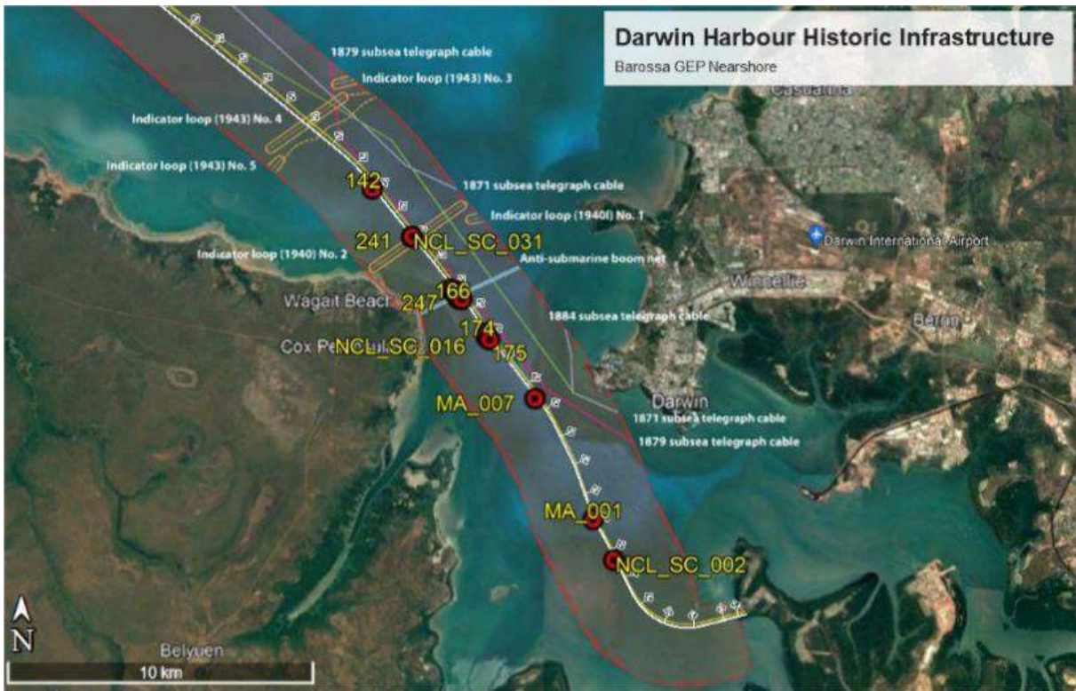
Figure 11-8 ROV survey target locations overlaid on a map of known historic maritime infrastructure in Darwin Harbour.
