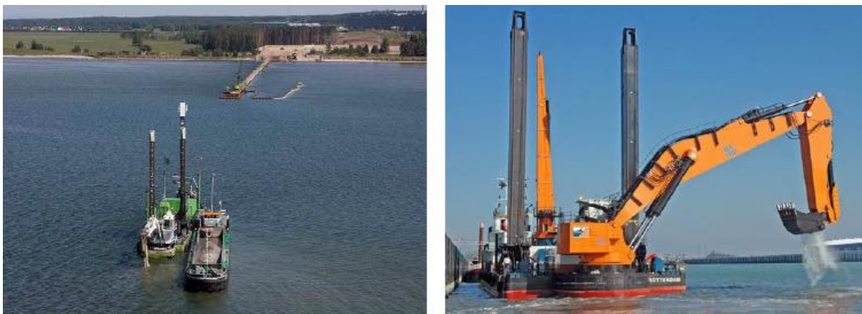
Figure 2-3: Typical Backhoe Dredgers (Dredging, Environmental and Marine Engineering (DEME) Offshore & Van Oord JV, 2022)
