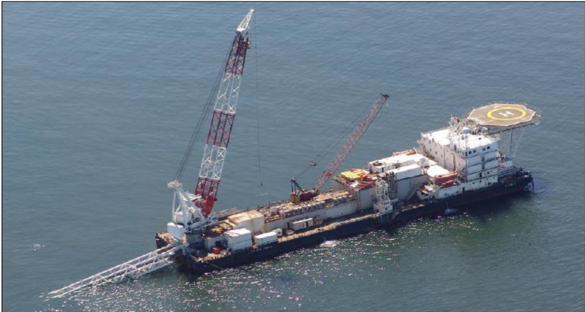
Figure 2-8: Example of pipelaying vessel (nearshore)
