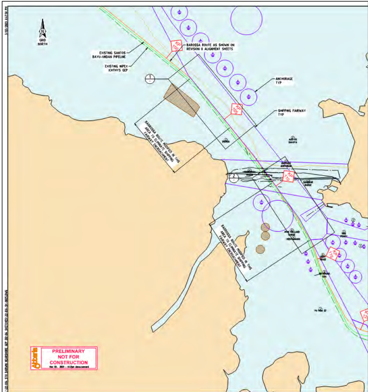
Figure 3-6 Section of the revised DPD pipeline northern route, following stakeholder engagement (option 2), showing reduced shipping channel encroachment
