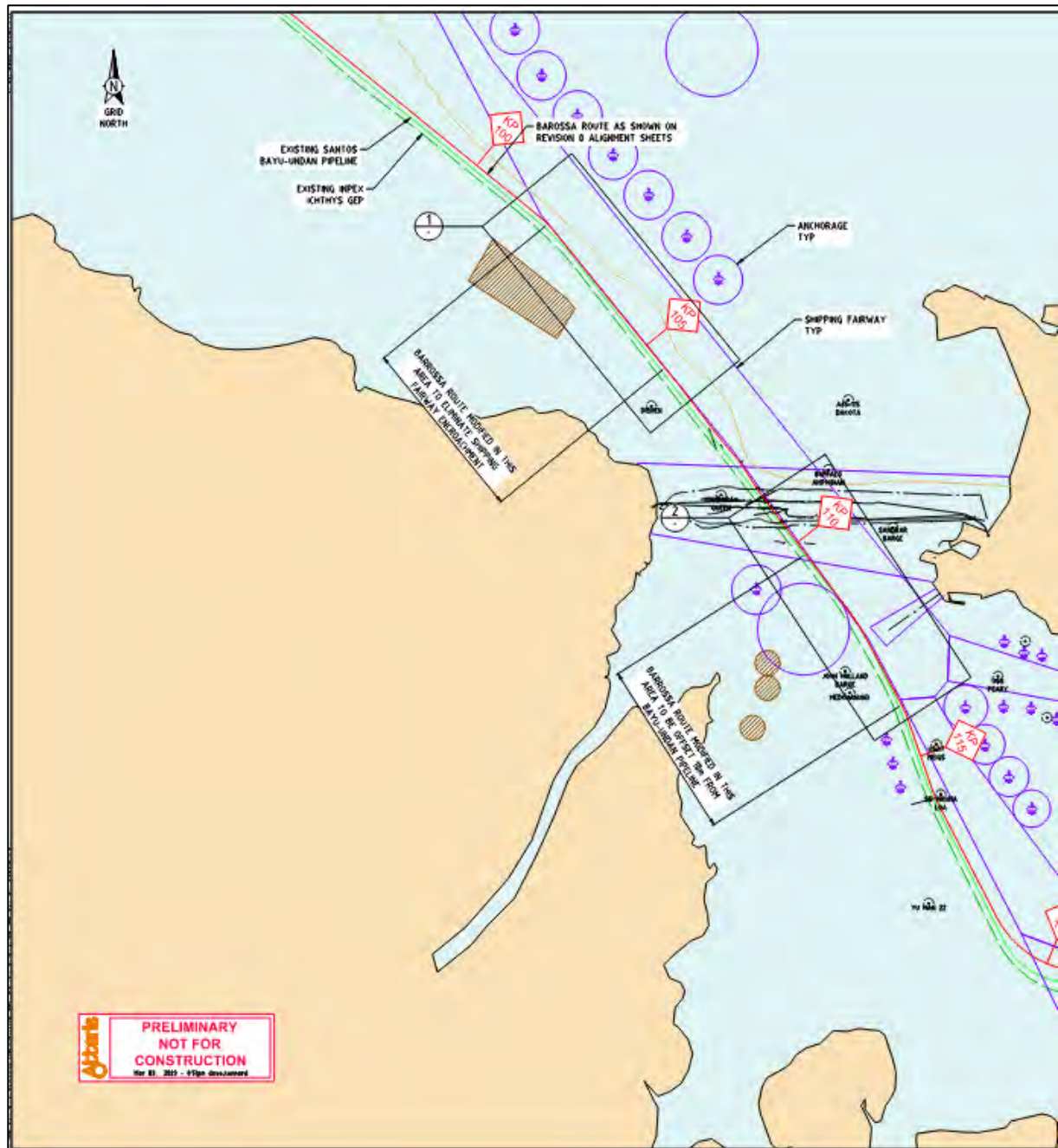
Figure 3-8 Section of the revised DPD pipeline northern route, following stakeholder engagement (option 3), showing removal of all shipping channel encroachment. This represents the final selected route.
