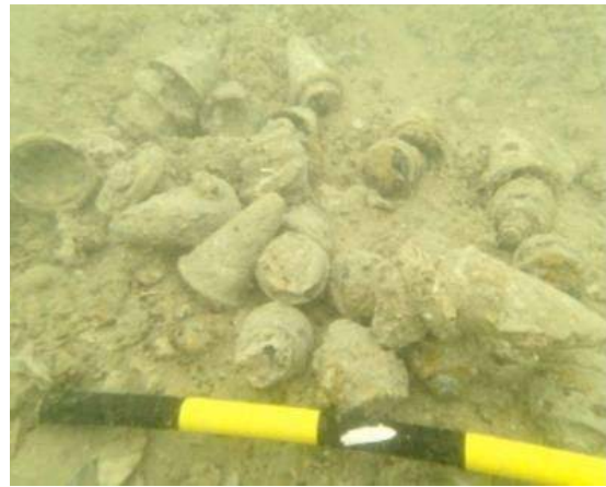
Figure 49: Collection of mechanical time fuses and fuse cones located at Contact 2. (Source: CA 2012).
