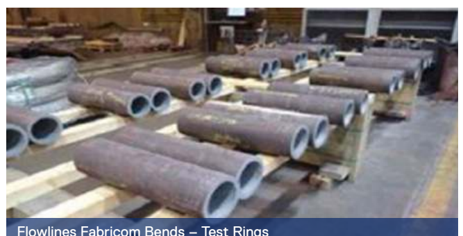
Flowlines Fabricom Bends – Test Rings
