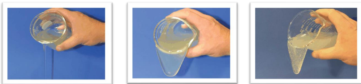
Figure 35: Example of Typical Stages of Gum (Guar) Cross-linking to Achieve 300 cp.
