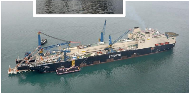
Dynamically positioned specialist pipelay vessel
