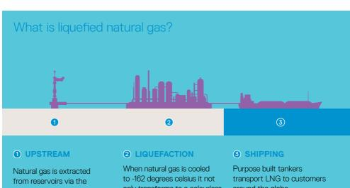
drilling of wells. This gas is then transported to a liquefaction facility through a pipeline network.
