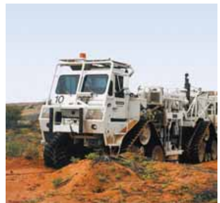
Vibroseis vehicles fitted with rubber tracts, which minimise land disturbance, acquiring seismic survey in the Cooper Basin.
