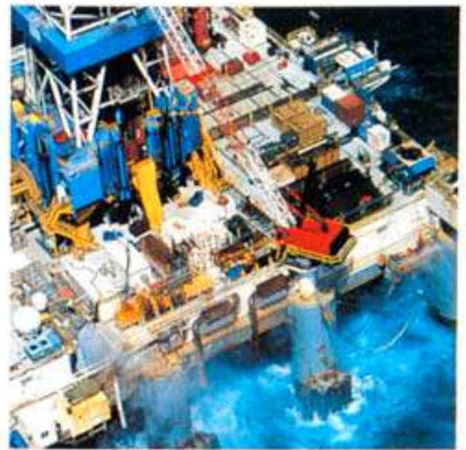
Timor Gap, Offshore Australia. The Atwood-Eagle, a semi-submersible rig drilling the successful Undan-1 well in ZOCA 91-12 during 1995.
