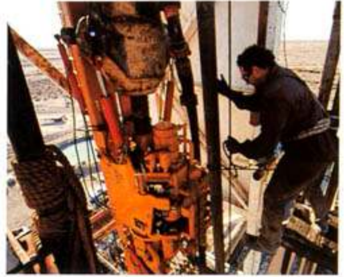
A drilling rig used in the Cooper/Eromanga Basins enhanced with new portable top drive technology.
