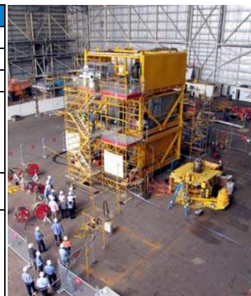
Wing deck module for John Brookes platform assembled for testing (subsea tree adjacent)
