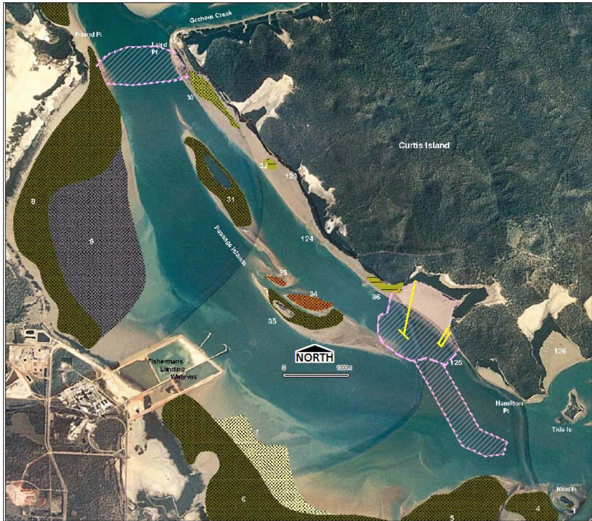
Key Area where dredge activities could generate underwater sound pressure levels up to 150 dB Area where pile driving activities could produce underwater sound pressure levels up to 150 dB msp Figure 6 Areas where temporary avoidance may occur during construction activities
