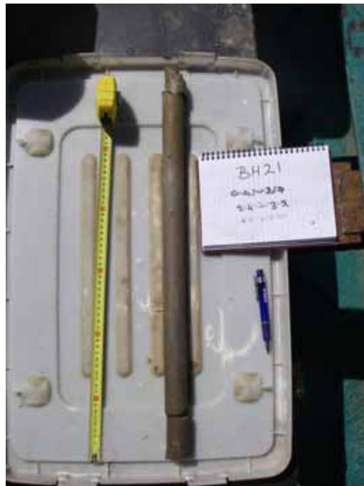
Plate 23: BH21 4.0-4.45 m (below seabed)
