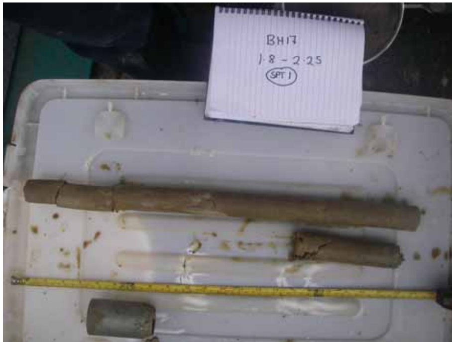
Plate 15: BH17 1.8-2.25 m (below seabed) SPT1
