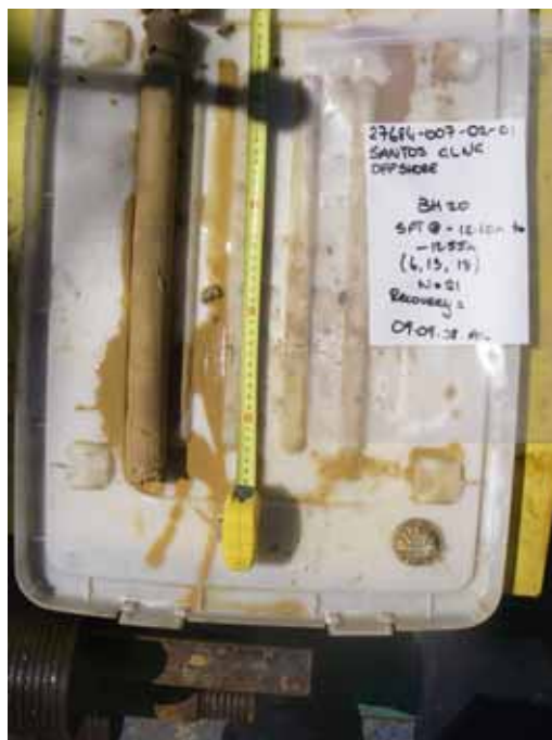
Plate 20: BH20 SPT @ 12.10 m (below seabed)
