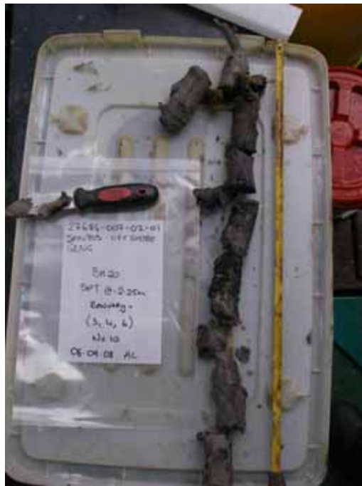
Plate 19: BH20 SPT @ 2.25 m (below seabed)
