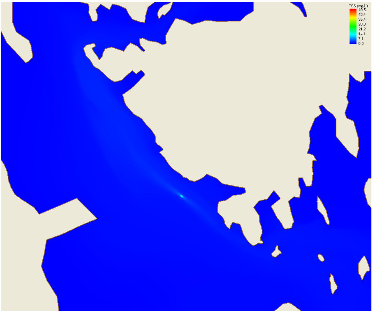
Figure 6-16 Average Total Suspended Solids Increases, Due to Capital Dredging Works - Spring Tide
