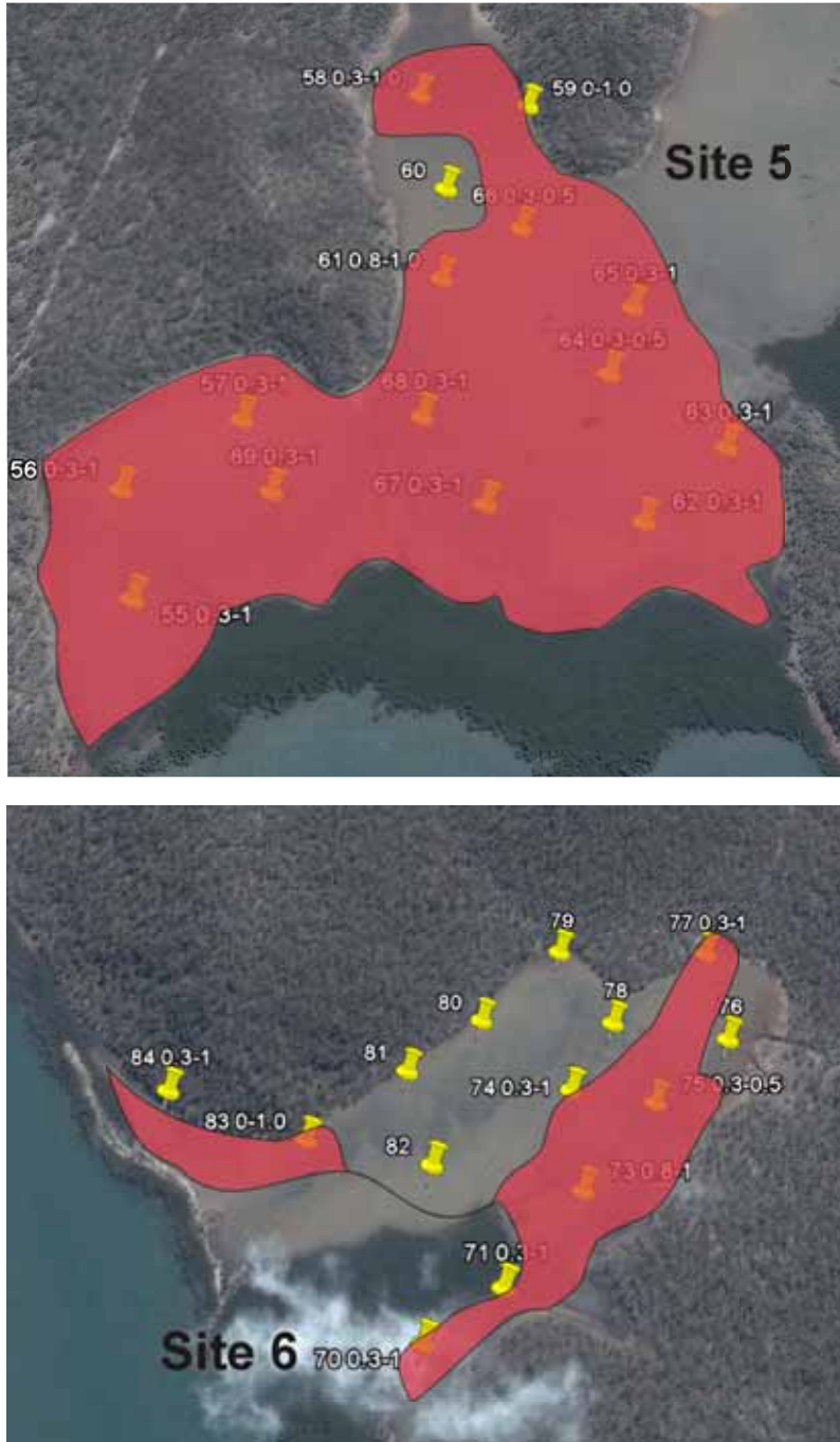
Figure D-1 Distribution of low but actionable levels of AASS ( >0.03\%S or 18 \text{ mol H}^+/\text{t} ) within the top 1 metre.
