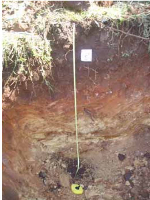
Plate A-11 Site #5, Group 7 soil (Type 7.1) – gradational gravelly clay soil in terrain unit Cw8/7.1
