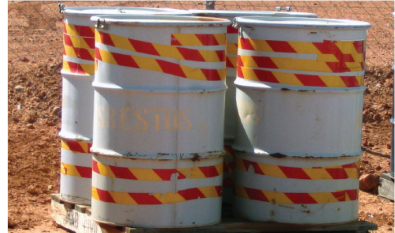
Asbestos in drums awaiting disposal.
