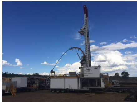
Savanna 407 coil tubing drilling rig executing Roma 3A drilling scope
