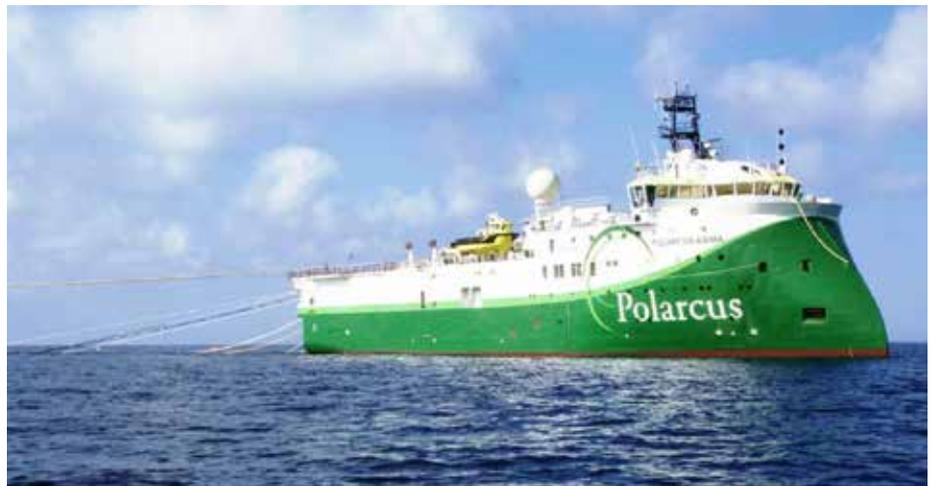
Figure 2: Polarcus Asima seismic survey vessel
